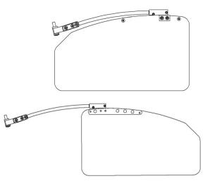
• To lengthen the effective reach, just rotate the visor 180° on its center pivot.
