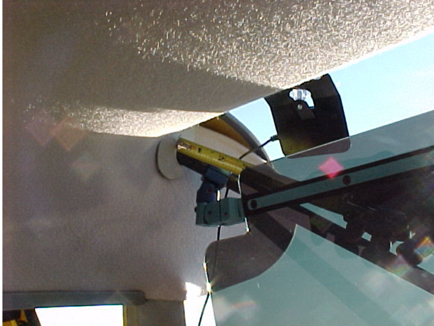
Maule Installation Example: Image showing measurement from corner soft goods
