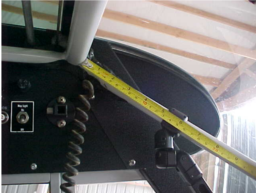
Husky Installation Example: Image showing measurement from cross tube.
