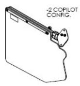
Orientate the mounting plate to find the most vertical position for the swivel. When installed the pivot post should be nearly vertical with respect to the aircraft.
