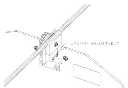
• After tensioning, install retaining e-clips PCS-1000-14S-STZ0 in the groove at the end of the thumb tension knob threads. **CAUTION**: Do not remove the tension knob once the e-clip has been installed, the visor clamping blocks will separate completely and become non-functional.
